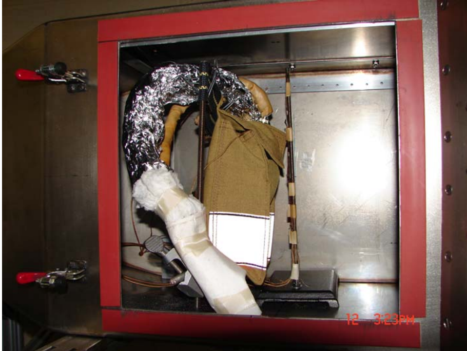
Figure 4 Pocket inside FEE for testing. Radio is inside with insulated cable attached. The speaker/microphone cable is the front cable with the aluminum foil at the top while the coax cable connecting the radio output to the spectrum analyzer is the back cable. A thermocouple tree is attached to the ring stand in front of the pocket and the airflow is from the left.
